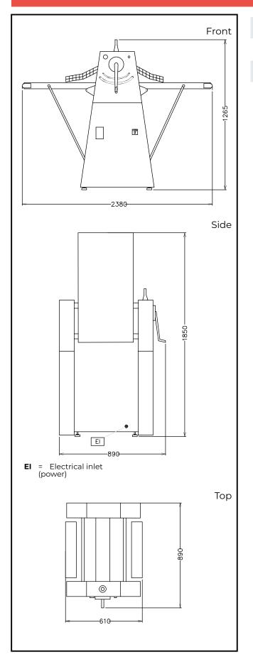
Electric Supply voltage: 230 V/1 ph/50/60 Hz 0.75 kW **Total Watts:** Key Information: External dimensions, Width: 2380 mm External dimensions, Depth: 890 mm External dimensions, 1265 mm Height: Net weight (kg): 179
